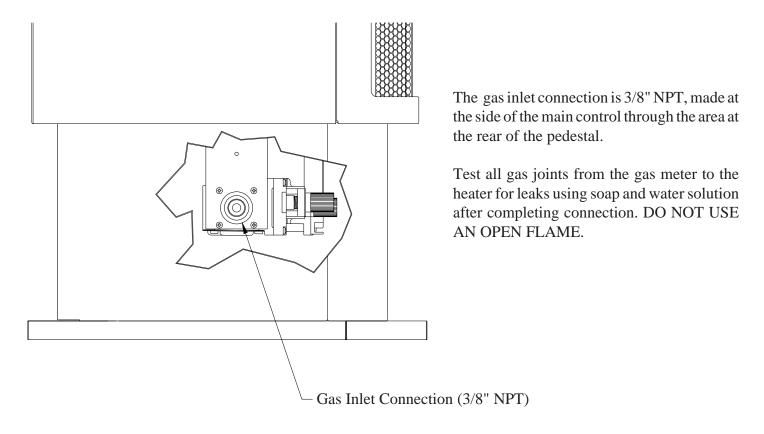
FIGURE 6. Rear View of 2045 Vent-Free Gas Heater
